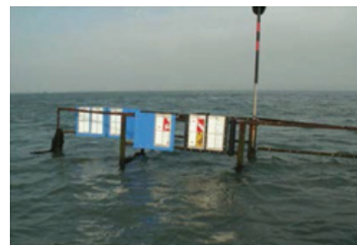
Actual third-party testing of Epson labels durability in marine immersion
