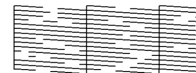
Example of clogged nozzles
