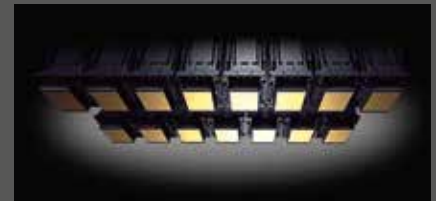
Epson Micro Piezo multi-printhead array
