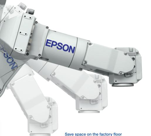
Replace with: Compared to conventional 6-axis robots, the ProSix N-Series robots require up to 75% less production space in production. Thanks to the completely new joint geometry with a foldable arm, they can reach every point of their work area without detours. They thus cover a field of action that would normally require a 6-axis machine with a significantly greater arm length.
