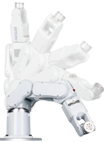
Saves space and reduces cycle times thanks to the possibilities for the axes 2 and 3 to rollover.
