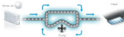
The pump circulates the white ink to prevent the printhead from clogging
