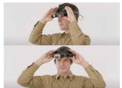
To flip up, hold the headband and push the display forward
