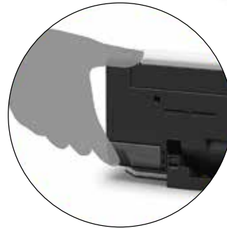
Sliding the position selector button across adjusts the scanner's angle
