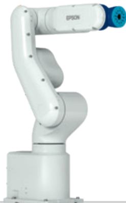
Epson ProSix-VT6-Series Payload: 6 kg Reach: 920 mm
