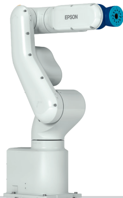
Epson ProSix-VT6-Series Payload: 6 kg Reach: 920 mm
