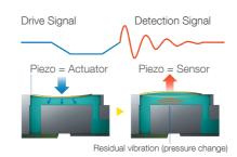
Ensure consistent, uninterrupted quality with Nozzle Verification Technology that detects blocked nozzles, and dot compensation that compensates for them.
