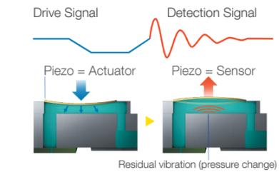
Ensure consistent, uninterrupted quality with Nozzle Verification Technology that detects blocked nozzles, and dot compensation that compensates for them. NVT works constantly behind the scenes to maximise reliability and reduce downtime.
